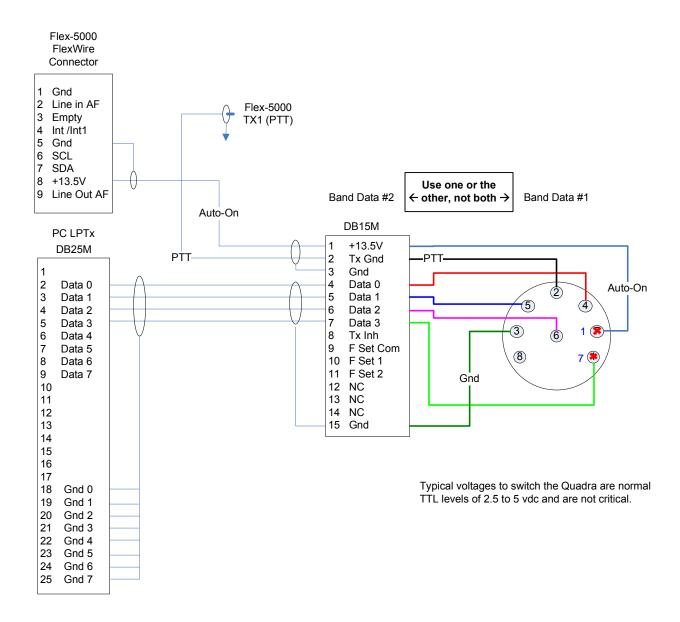
Please note that the connections for the Band Data 1 are **un-proven** but are thought to be correct. It is known that the Band Data 1 connection information from the Yaesu Quadra manual is **incorrect** in at least some instances. So proceed with caution until the Band Data 1 connection information is verified.
